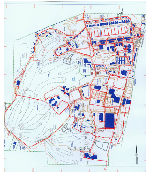
Figure 2-15 Existing Water Supply System
